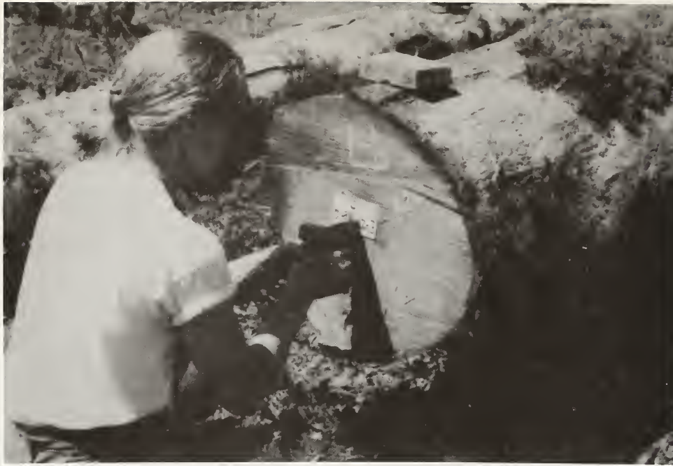
Maintaining the identity of logs, such as this red alder, is a critical part of mill recovery studies.
